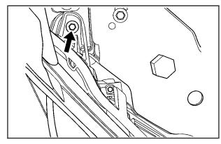
2. Remove the screw from the headlamp assembly.
